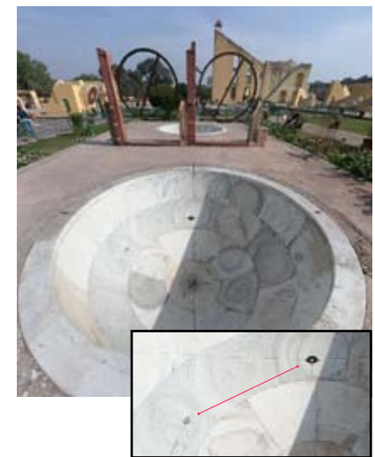
The Kapala A at Jaipur. The crosswire, center plate, and its shadow can be clearly seen in the inset.
