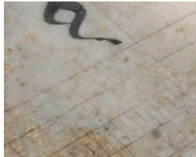
Time subdivisions on the quadrant scale. The smallest subdivisions, visible in the lower right corner, represent intervals of two seconds.
